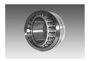
The following bearings are designed for use in mobile cement mixer gearboxes. The bearings are mounted onto the main shaft of the gearbox and are offered in three basic designs: PLC 58-6, PLC 59-5, and PLC 59-10, all have a wider outer ring, increasing the self-aligning ability of the bearing. These bearings are produced within ABEC 1 tolerance and have a C0 radial clearance.
