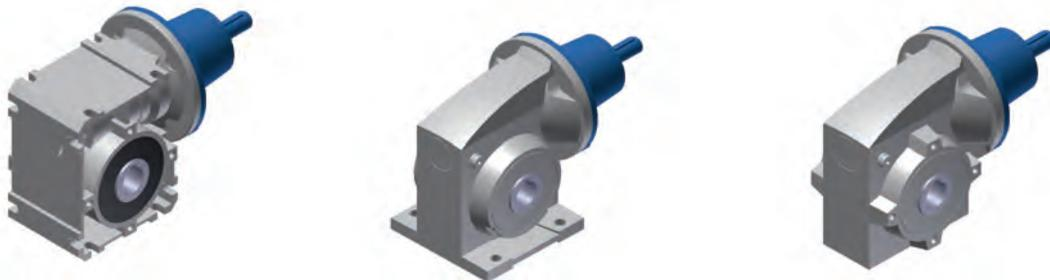
The Type W free input shaft was developed to attach couplings, belt pulleys or chain wheels to the input of NORD UNIVERSAL worm gear units. The Type W free drive shaft is available for sizes 40, 50, 63 and 75. The components includes the pre-assembled, lubricated-for-life unit, the coupling sleeve and all the necessary fastening elements.
