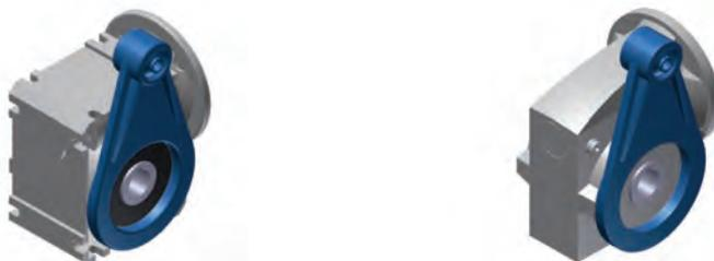
The torque support is a compact and simple method for absorbing reaction torques with shaft-mounted gear units. The torque support is mounted on the B14 threaded holes of the NORD UNIVERSAL worm gear unit and can be installed with rotation steps of 45°.
