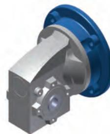
Short, compact motor mounts enable the attachment of standard IEC motor sizes from 56 to 112 or NEMA standard motors from 48C to 184TC
