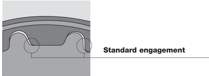
To improve transmission precision, it is possible to use zero or reduced backlash pulleys. Please note that these pulleys don't reduce the elasticity of belt teeth or cords.
