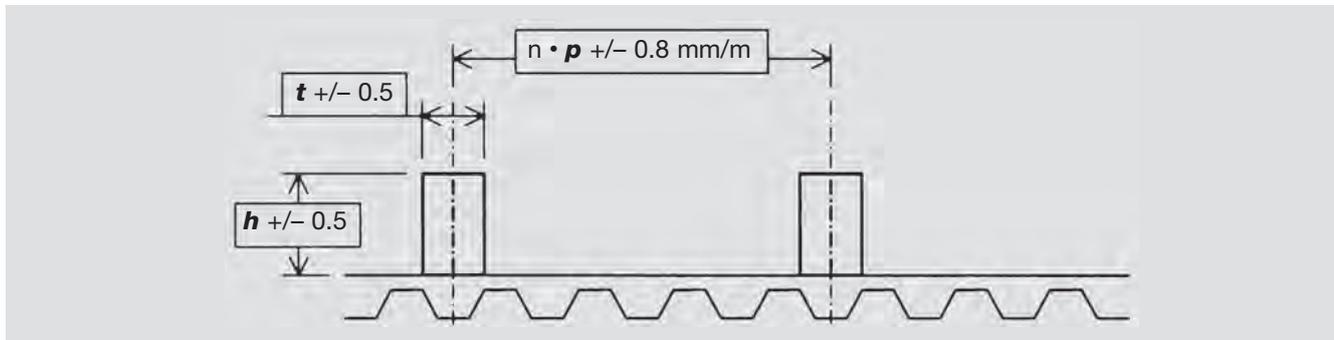
The tolerances on the position are +/- 0.5 mm.
