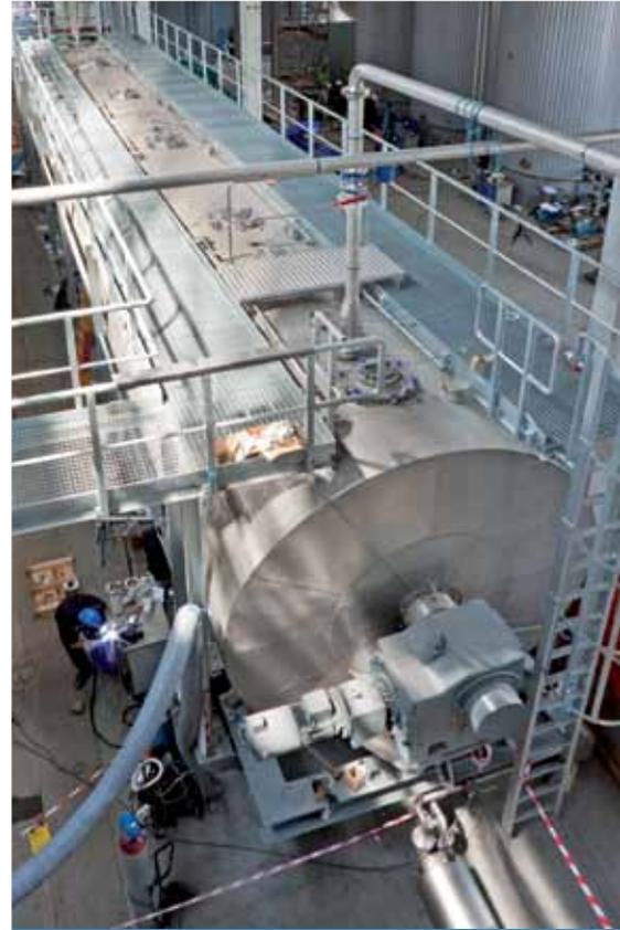
Powerful bevel geared motors mounted in pairs on the mixing drums deliver maximum output torques of over 53,000 Nm.
