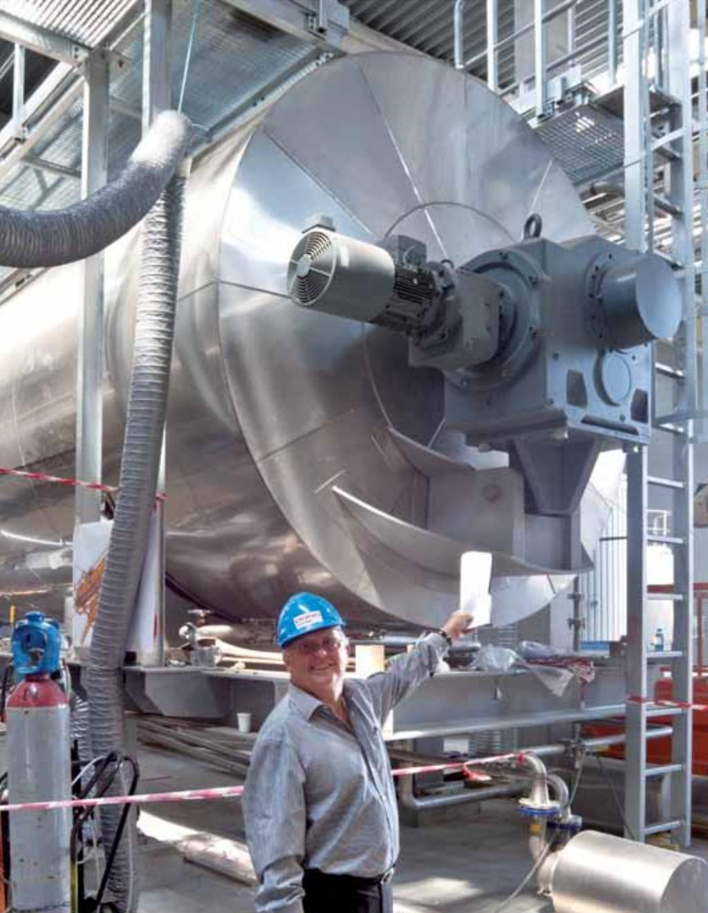
In four 20 m long mixing drums, movement is provided by bevel geared motors mounted in pairs on the longitudinal shaft.
