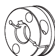
Type 2.6 Clamping hub double slot, with feather keyway Positive locking power transmission with additional frictionally engaged condition. The frictionally engaged condition prevents or reduces reverse backlash, respectively. Surface pressure of the keyway connection is reduced.
